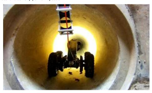
Municipal drainage network is one of the important infrastructure of the city, in urban life, the drainage network is as indispensable as the blood vessels of the human body, and the installation of pipes in the construction of the network is an important hidden project, is the core of the quality of the entire project, pipeline inspection robot to drainage network inside the peep detection is good to grasp the pipeline situation.
